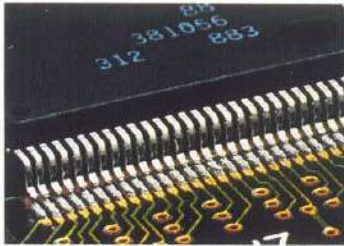
The LSM makes it possible to verify the quality of solder paste printing on critical fine-pitch sites.
