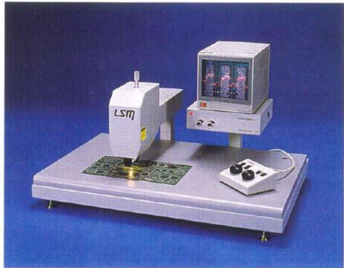
LSM measures fine pitch solder paste.
