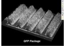
The **AP2/2** allows operators to obtain 3D color profiles for fast and accurate paste analysis. Operators may use these profiles to help them determine what corrections are needed in their solder paste printing process, thereby improving yields.
